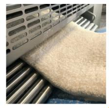
The Rijkaart 4 roll dough band former is a reliable and trusted head machine for the Rijkaart bread line. The 4 adjustable rollers give extreme control over the structure and weight consistency of the dough band.
