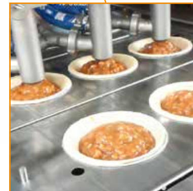
servo depositing is 30% more accurate than pneumatic systems
