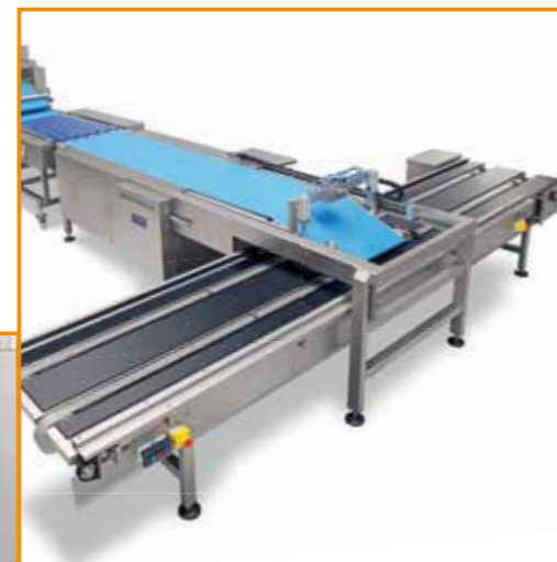
After the products are cut, they are transported to the nose of the retracting system. After being sensed by a photo eye, the retractor travels to the back position and the products are transported to the below conveyor.
