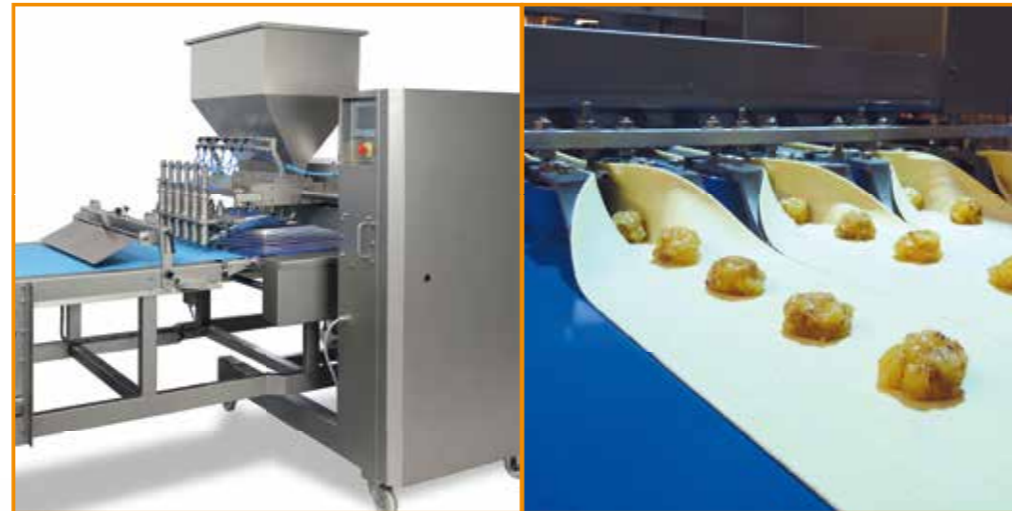
Rijkaart servo driven spot depositor and folding plow system produces a variety of filled and folded products
