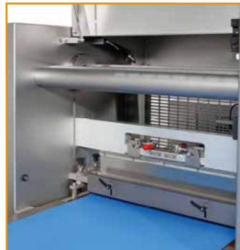
After the products are cut, they are transported to the nose of the retracting system. After being sensed by a photo eye, the retractor travels to the back position and the products are transported to the below conveyor.
