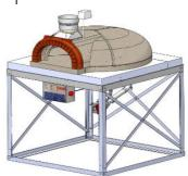
Including: oven 950 or 1030 - Hooping -Flue connector-cast iron door-vault insulation of mineral wool- floor insulation of cecalu-1 burner 27 kW - 1 ignition kit and check kit- 1 depression monitoring of the pipe - 1 security to avoid a overheating of the vault-1 probe to measure the temperature of the floor- 1 box with device to check and automate the gas mechanism-1 reinforced support- 1 hood made of resin or inox plate.
