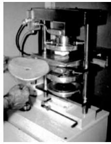
3. Remove finished bottom crust from Press, finished top crust on polyfilm sheet.
