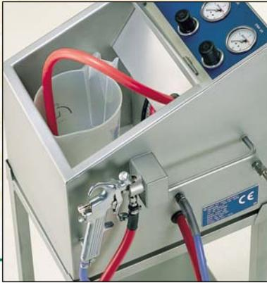
Whilst we are constantly improving our machines to the requirements of the users, we have developed the Chocospray 100: a machine, which sprays chocolate (coating) directly from an (open) heated reservoir. This reservoir is heated by means of a hot-air circulation, where the temperature can be adjusted digitally. With the introduction of the electrically heated chocolate spraying hose blockages are a thing of the past.
