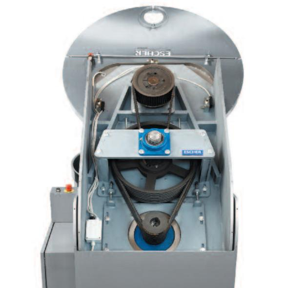
The new taper bowl locking and motion system is technically superior to the traditional systems as it utilizes a taper coupling to join the machine and the trolley. The trolley is locked by means of a taper shaft that, as it ascends, centres the bowl and moves it into the working position.
